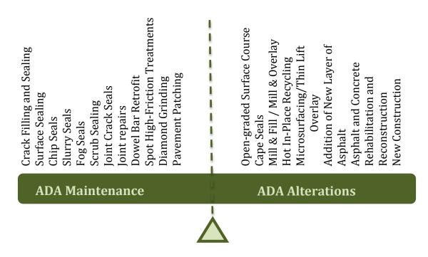
This approach clearly identifies the types of structural treatments that both DOJ and FHWA agree require curb ramps (when there is a pedestrian walkway with a prepared surface for pedestrian use and a curb, elevation, or other barrier between the street and the walkway) and furthers the goal of the ADA to provide increased accessibility to the public right-of-way for persons with disabilities. This single Federal policy will provide for increased consistency and improved enforcement.
